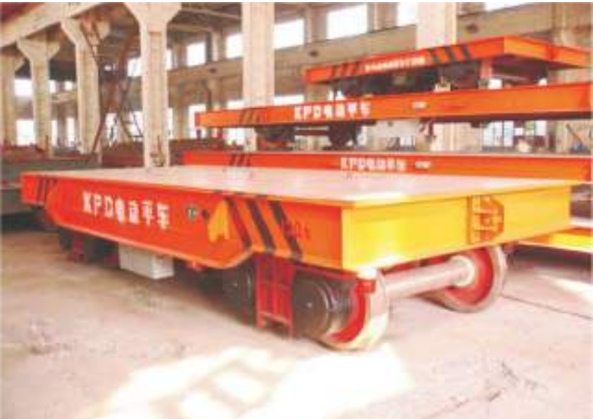
Rail Transfer Cart
