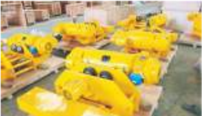
Low Clearance Hoist
