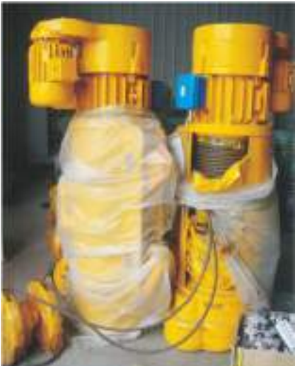
Dual Speed Electric Hoist
